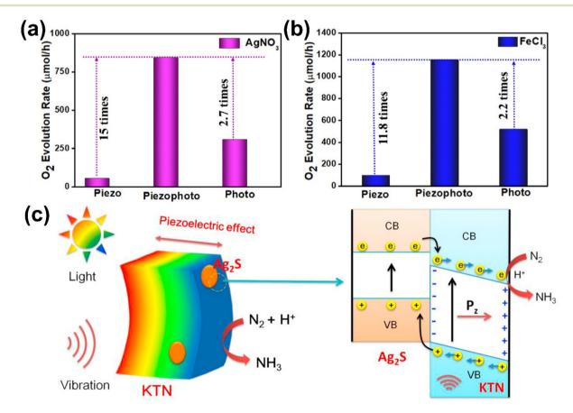
Fig. 14 (a and b) Photo-piezocatalytic oxygen evolution rates over NaNbO<sub>3</sub>/FeOOH in the presence of (a) AgNO<sub>3</sub> and (b) FeCl<sub>3</sub> as sacrificial agents. Reprinted with permission from ref. 154. Copyright 2023, American Chemical Society. (c) Schematic illustrations showing the mechanism of photopiezocatalytic N<sub>2</sub> fixation over Ag<sub>2</sub>S/KTN heterojunction. Reprinted with permission from ref. 160. Copyright 2023, Elsevier.
