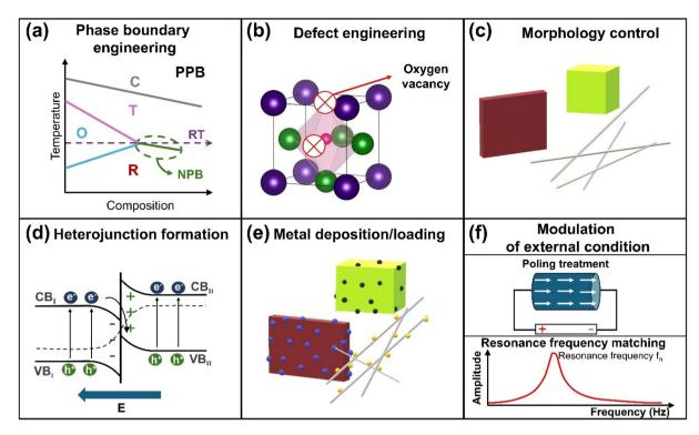
Fig. 4 Design strategies for improving piezocatalytic and photo-piezocatalytic activities of KNN-based materials. ((a) Phase boundary engineering, (b) Defect engineering, (c) Morphology control, (d) Heterojunction formation, (e) Metal deposition/loading, and (f) Modulation of external condition.
