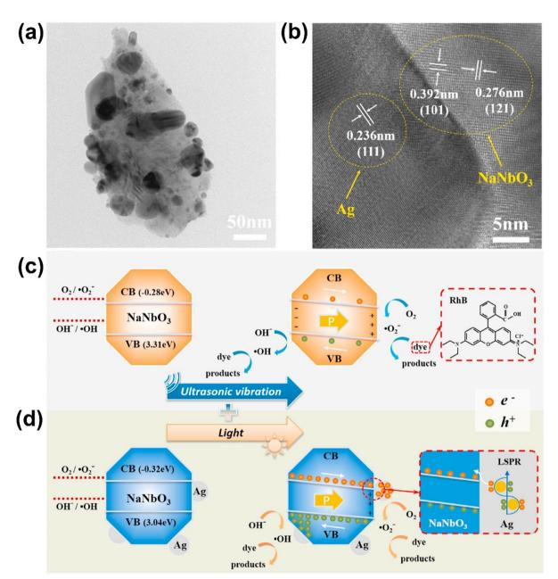
Fig. 11 (a) TEM and (b) HR-TEM images of Ag dot decorated NaNbO<sub>3</sub>. (c and d) Possible mechanism of piezocatalytic and photo-piezocatalytic dye degradation of Ag/NaNbO<sub>3</sub>. Reprinted with permission from ref. 133. Copyright 2022, Elsevier.
