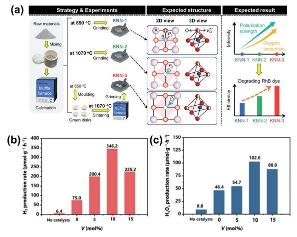
Fig. 13 (a) Schematics on experimental procedures, expected structures, and properties of three different KNN materials prepared by applying different calcination and sintering conditions. Reprinted with permission from ref. 145. Copyright 2024, Wiley. (b) Piezocatalytic H<sub>2</sub> and (c) H<sub>2</sub>O<sub>2</sub> production rates of V-doped NaNbO<sub>3</sub> samples with different V doping. Reprinted with permission from ref. 150. Copyright 2022, Springer.
