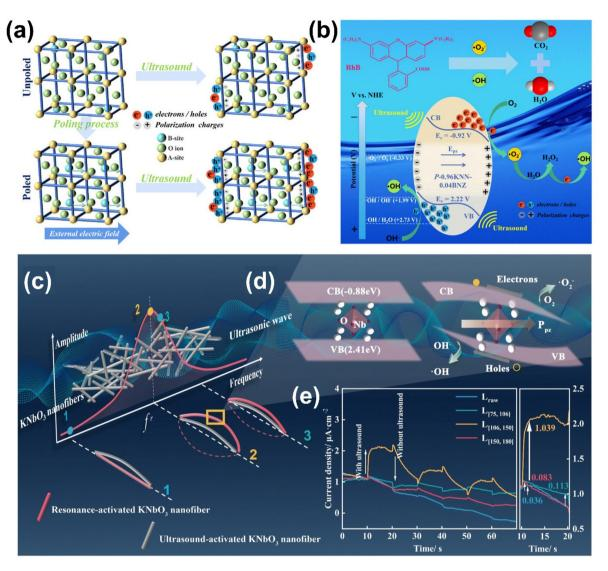
Fig. 12 (a) Schematic drawings of poling and ultrasound actions on KNN-BNZ ceramics. (b) A possible mechanism of piezocatalytic dye degradation using polarized KNN-BNZ ceramics. Reprinted with permission from ref. 138. Copyright 2024, Wiley. (c) Resonance-induced deformation and (d) band structure variation of KNbO<sub>3</sub>. (e) Current density of KNbO<sub>3</sub> with different natural frequencies at 30 kHz. Reprinted with permission from ref. 140. Copyright 2024, Royal Society of Chemistry.
