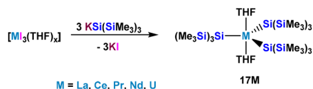
Scheme 3 Synthetic access to a number of trisilylated ate-complexes 17M .
