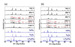
Fig. 2 XRD patterns of (a) sample A and (b) sample D after heating for 30 min at 750, 850, 950, 1050, and 1100 °C. Bottom: Simulated reference patterns based on ICSD for TaPO $_5$  (#202041), Ta $_2$ O $_5$  (#9112), and LiTa $_2$ PO $_8$  (#110781). The peaks indicated by red circles are attributed to LTPO-Precursor in this study.
