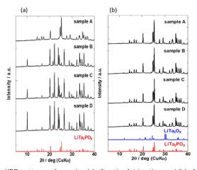
Fig. 3  $\,$  XRD patterns of samples (a) after the 1st heating and (b) after the 2nd heating. Bottom: Simulated reference patterns based on ICSD for LiTa<sub>3</sub>O<sub>8</sub> (#493) and LiTa<sub>2</sub>PO<sub>8</sub> (#110781).
