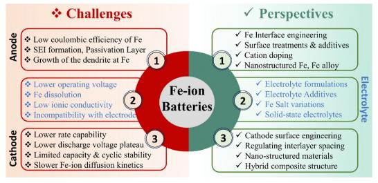
Fig. 11 Challenges and corresponding perspectives related to the different components of rechargeable Fe-ion batteries.
