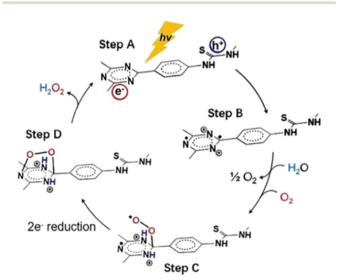
Fig. 13 Mechanism for photocatalytic  $H_2O_2$  production on the surface of Bpt-CTF. Adapted with permission from ref. 145. Copyright 2022 Wiley.
