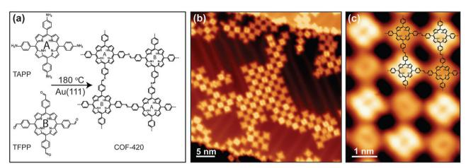
Fig. 5 (a) Schematic representation of the synthesis of COF-420 from the molecular precursors TAPP and TFPP. (b) Representative large-scale STM topographic image of COF-420 on Au(111) (sample bias  $V_s = 0.8 \text{ V}$ , tunnel current  $I_t = 10 \text{ pA}$ ). (c) Close-up STM image of COF-420 with the chemical structure overlaid in the top-right corner ( $V_s = 0.8 \text{ V}$ ,  $I_t = 10 \text{ pA}$ ). Adapted with permission from ref. 94. Copyright 2019 Wiley.
