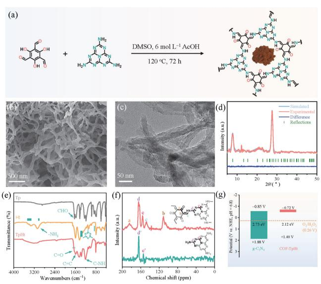
Fig. 12 (a) Schematic synthetic protocol towards COF-TpHt together with its molecular structure and photograph of the powder product. (b) SEM imaging. (c) TEM imaging. (d) Experimental and simulated XRD patterns of COF-TpHt together with its structural refinement. Adapted with permission from ref. 137. Copyright 2023 Elsevier.
