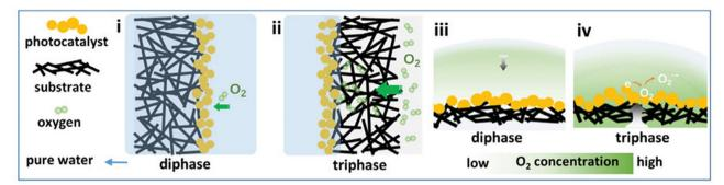
Fig. 14 Schematic illustration of diphase and triphase photocatalytic conditions. Adapted with permission from ref. 146. Copyright 2021 Wiley.
