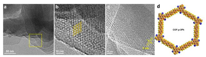
Fig. 7 (a) TEM image of COF-p-3Ph. (b) Enlarged view of a selected area in the panel (a). The structural model is overlapped on the top. (c) TEM image of COF-p-3Ph from a different area, showing 1D channels with a width of 3 nm. (d) Illustrative structure of COF-p-3Ph. Adapted with permission from ref. 104. Copyright 2019 American Chemical Society.
