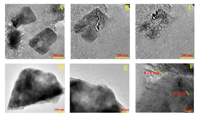
Fig. 4 TEM images of the 2:1 Co-Fe-MOF showing the cuboidal type morphology (A) and subsequent disintegrations (B) and (C). TEM (D) and (E) and HR-TEM (F) images after the OER catalysis of the 2:1 Co-Fe-MOF.
