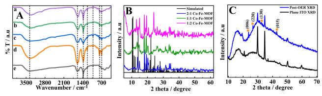
Fig. 1 FT-IR spectra (A) of the 2:1 Co-Fe-MOF (a), 1:1 Co-Fe-MOF (b), 1:1 Co-Fe-MOF (c), Co-MOF (d), and Fe-MOF (e) and the powder XRD pattern (B) and post-catalysis XRD pattern of the 2:1 Co-Fe-MOF (C).
