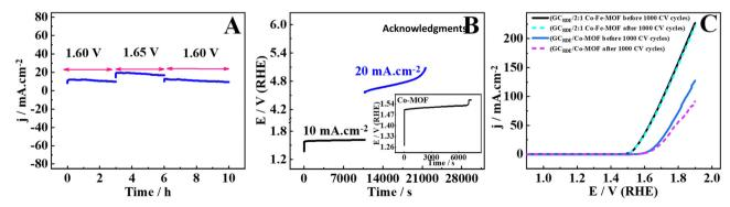
Fig. 7 Stability tests for the 2:1 Co-Fe-MOF and Co-MOF via amperometry (A), chronopotentiometry (B), and LSV response before and after 1000 CV cycles (C).
