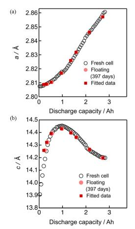
Fig. 8 Least squares fitting results of the lattice constants (a) a and (b) c for the cell after 397 days of floating
