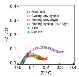
Fig. 4 Nyquist plots of fully charged before and after durability test.
