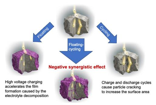
Film formation within the cracked particles significantly limits the ion transportation paths
