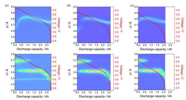
Fig. 6 Neutron diffraction patterns of 003 diffraction of positive electrode (upper) and 00*l* diffraction of negative electrode (lower): (a) fresh cell, (b) floating-cycling after 160 days, (c) floating-cycling after 397 days.
