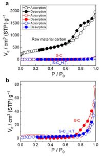
Fig. 3 (a) The N<sub>2</sub> adsorption/desorption isotherms of the raw material carbon, S-C and S-C\_H.T. (b) The enlarged N2 adsorption/desorption
