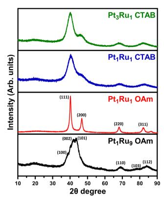
XRD data for all of the alloyed samples generated
