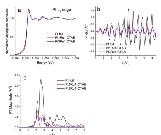
Fig. 4 (A) Pt  $L_3$ -edge XANES data. (B)  $k^2$ -weighted EXAFS data in k-space. (C) Fourier transform magnitudes of the  $k^2$ -weighted EXAFS data for Pt foil, Pt<sub>1</sub>Ru<sub>1</sub> (produced with CTAB), and Pt<sub>3</sub>Ru<sub>1</sub> (produced with CTAB).
