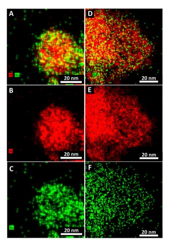
Fig. 2 EDS elemental maps of PtRu generated using the CTAB method. Pt<sub>1</sub>Ru<sub>1</sub> maps are provided as follows: (A) the composite of Pt and Ru, (B) Pt, and (C) Ru. Analogous Pt<sub>3</sub>Ru<sub>1</sub> maps are shown, as (D) the composite of Pt and Ru, (E) Pt, and (F) Ru.
