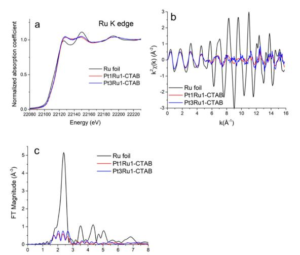
(A) Ru K-edge XANES data. (B)  $k^2$ -weighted EXAFS data in k-space. (C) Fourier transform magnitudes of the  $k^2$ -weighted EXAFS data for Ru foil, Pt<sub>1</sub>Ru<sub>1</sub> (produced with CTAB), and Pt<sub>3</sub>Ru<sub>1</sub> (generated with CTAB).
