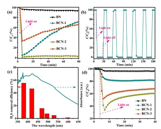
Fig. 6 (a) Photocatalytic  $H_2S$  removal activity of all the samples, (b) photocatalytic activity testing of the BCN-2 sample under light on-off cycles, (c) photocatalytic activity testing of the BCN-2 sample under different monochromatic wavelengths and (d) photocatalytic NO purification of all the samples.
