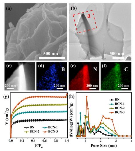
Fig. 3 (a) SEM image of the BCN-2 sample, (b) TEM image of the BCN-2 sample, (c-f) element mapping images of the BCN-2 sample, (g)  $N_2$  adsorption-desorption isotherm plots of all samples and (h) the pore size distribution of all samples.
