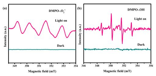
Fig. 8 DMPO EPR spin-trapping of the BCN-2 sample for  ${}^{\bullet}O_2^-$  (a) and  ${}^{\bullet}OH^-$  (b) radicals.
