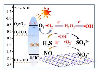
Fig. 9 Schematic of photocatalytic removal of gas contaminants over the BCN catalyst.
