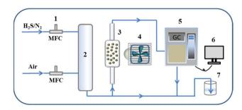
Scheme 1 Schematic diagram of the photocatalytic  $H_2S$  removal process. (1) Mass flow controller; (2) gas mixing tank; (3) reactor; (4) light source; (5) gas chromatograph; (6) computer; (7) tail gas collector.
