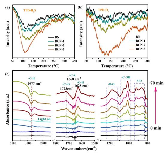
Fig. 7 (a) The temperature-programmed desorption curves of  $H_2S$  for all the samples, (b) the temperature-programmed desorption curves of  $O_2$  for all the samples, (c) DRIFTS test for photocatalytic  $H_2S$  removal over the BCN-2 sample.
