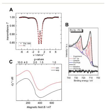
Fig. 5 Zero-field <sup>57</sup>Fe Mössbauer spectrum of Fe-HBC-MOF recorded at 77 K in the solid state (A), XPS spectrum of the Fe 2p region (B) and CW X-band EPR spectrum recorded at 293 K (C).
