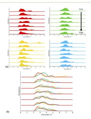
Fig. 7 (a) Plots of the pore size distributions calculated after network generation and desolvation for each solvent summed over each respective solvent models. (b) Comparison of the different solvent model pore size distributions. Stacked with increasing distance from the cluster edge to the core. Key: toluene – blue, THF – yellow, 1,4-dioxane – green, DMF – red.
