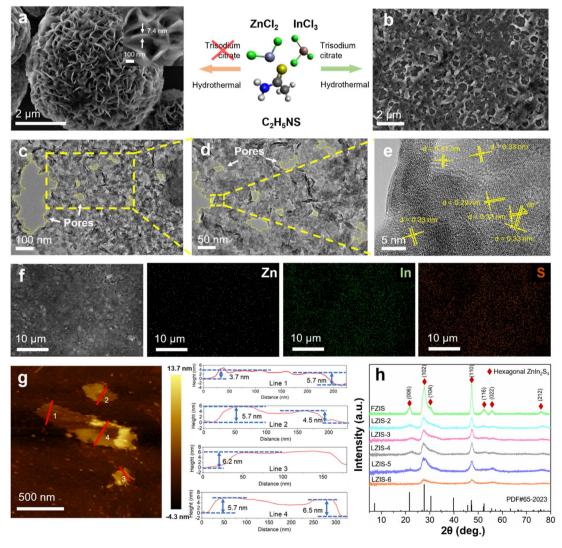
Fig. 1 FESEM images of (a) pristine ZnIn<sub>2</sub>S<sub>4</sub> nanoflowers and (b) LZIS-4. The inset of (a) depicts the thickness of the pristine ZnIn<sub>2</sub>S<sub>4</sub> nanoflowers. (c and d) TEM and (e) HRTEM images of LZIS-4. (f) FESEM-EDX mapping images of LZIS-4, where white, green and red represent Zn, In and S, respectively. (g) AFM topographic image and the corresponding height profiles of LZIS-4. (h) XRD of the as-prepared ZnIn<sub>2</sub>S<sub>4</sub> samples.
