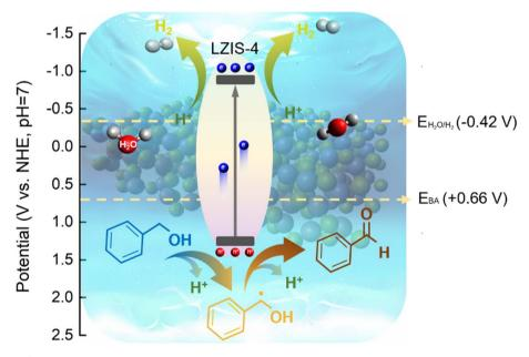
Fig. 7 A schematic of LZIS-4 in the dual coupling reaction of H<sub>2</sub> evolution and benzyl alcohol oxidation.
