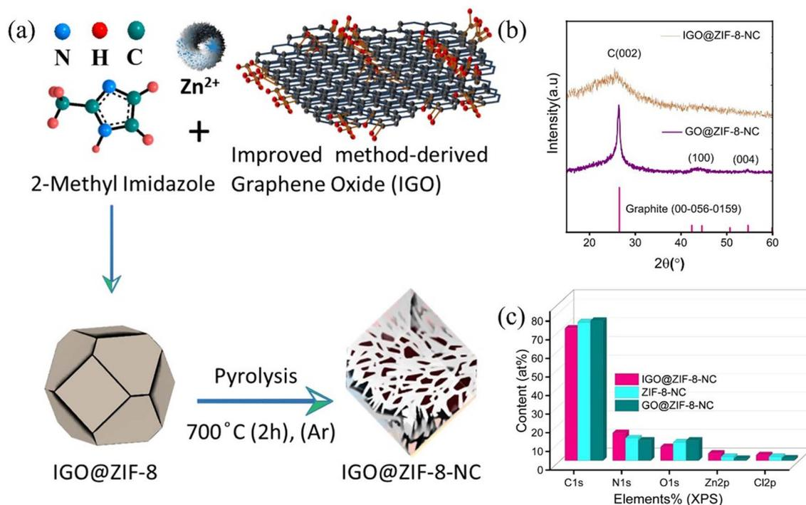
**Fig. 1** Schematic illustration of the synthesis process of the nanoporous N-doped carbon framework (IGO@ZIF-8-NC) by using the IGO, metal ion and linker. (b) XRD of IGO@ZIF-8-NC and GO@ZIF-8-NC, and (c) elemental atomic content of each element in various samples based on ESI Table 1 results calculated from XPS survey spectra.
