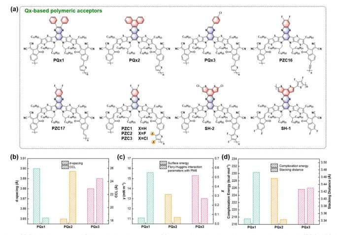
Fig. 6 (a) Chemical structures of Qx-based polymeric acceptors. (b)  $\pi - \pi$  stacking d-spacing and crystalline coherent length (CCL) of PQx1, PQx2, and PQx3 neat films. (c) Surface energy of the three polymeric acceptors and the Flory-Huggins interaction parameters with PM6. (d) Complexation energy and stacking distances of three polymeric acceptors with PM6 according to the theoretical calculation. Reproduced from ref. 64 with permission from Wiley, copyright [2023]
