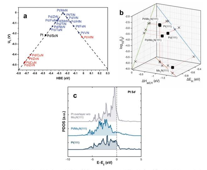
Fig. 7 (a) Volcano relationship for Pt-modified TMNs. (b) Correlation between the HER activity ( $log_{10}(i_0)$ ) and the binding strength of atomic hydrogen determined by TPD ( $\Delta H_{ad,H}$ ) and DFT ( $\Delta E_H$ ). (c) Projected density of states (PDOS) for Pt and Pt/TMN surfaces. (a) Reprinted from ref. 114 with permission from the Royal Society of Chemistry, Copyright 2022. (b and c) Reprinted from ref. 37 with permission from the American Chemical Society, Copyright 2023.
