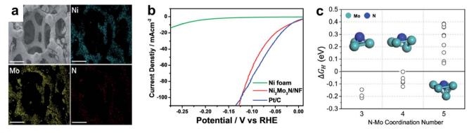
Fig. 9 (a) SEM-EDS of Ni<sub>2</sub>Mo<sub>3</sub>N/NF with scale bar of 300  $\mu$ m. (b) LSV curves of Ni foam, Ni<sub>2</sub>Mo<sub>3</sub>N/NF, and Pt/C in 1.0 M KOH electrolyte. (c) The Gibbs free energy of adsorbed hydrogen ( $\Delta G_H$ ) on different nitrogen adsorption sites with varying coordination number for N-Mo bonding. Reprinted from ref. 141 with permission from the Royal Society of Chemistry, Copyright 2021.
