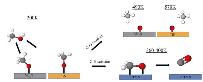
Fig. 3 Schematic representation of reaction pathways for methanol on  $Mo_2N$  and TiN. An inclined methoxy intermediate was formed on  $Mo_2N$  while a perpendicular orientation was taken on TiN. C–H bond scission to form CO was favored on 1 monolayer (ML) Pt-covered surfaces and C–O bond scission was suppressed.
