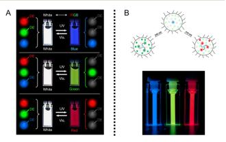
Fig. 5 (A) The photoswitching fluorescence of a mixed solution based on the combination of three distinct types of PF NPs.<sup>40</sup> Adapted with permission from ref. 37. Copyright 2014 Springer Nature. (B) Scheme of multiple-emission in single PF NPs.97 Adapted with permission from ref. 92. Copyright 2019 Springer Nature.
