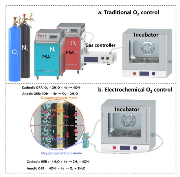
Working mechanisms of different  $O_2$ -control methods: (a) traditional  $O_2$ -control method, and (b) electrochemical  $O_2$ -control method.
