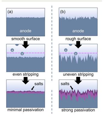
Fig. 6 (a) An even electric field leads to smooth metal stripping, while (b) an uneven electric field caused by surface heterogeneities leads to nucleation of metal salts as the anode is oxidized.
