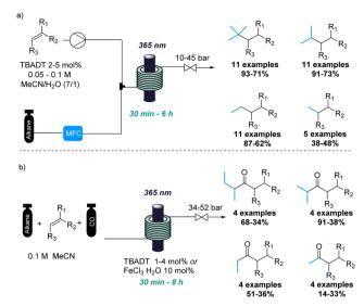
**Scheme 2** Flow intensification activating light alkanes *via* photocatalysis.
