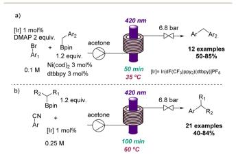
Scheme 8 Photochemical C(sp<sup>2</sup>)-C(sp<sup>3</sup>) cross-coupling reactions in flow
