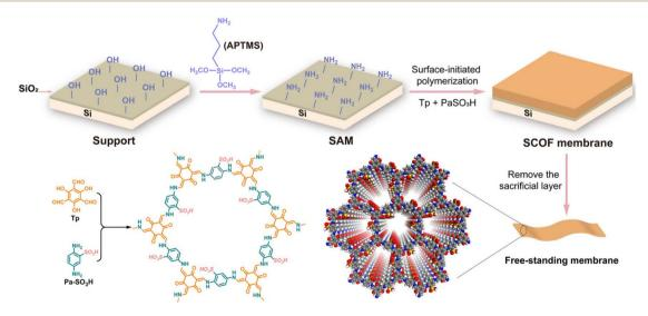
Fig. 5 Schematic route for the preparation of the SCOF membrane grafted on silicon wafers and the free-standing SCOF membrane, molecular structures of Tp,  $Pa-SO_3H$  and  $TpPa-SO_3H$ . Copyright 2021 Wiley-VCH GmbH.
