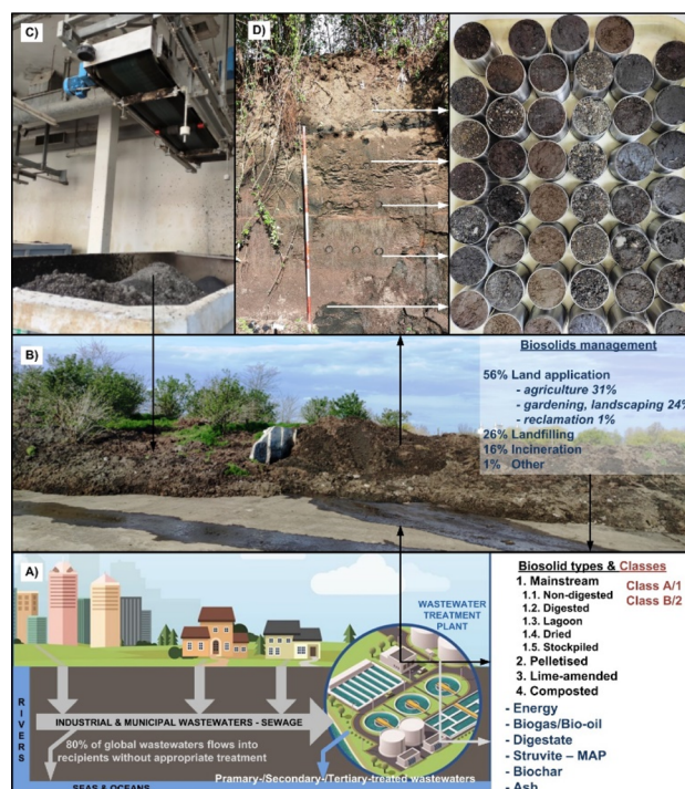
Fig. 2 Schematic presentation of a wastewater treatment plant as a resource of biosolids (BS) and value-added (co)products (A). Sewage sludge landfill at Zagreb Wastewater Ltd (B). Liming of fresh sewage sludge (C). Sampling of aged sewage sludge in undisturbed conditions (D). Reproduced (adapted) with permission from ref. 32. Copyright© 2023, Uni. of Zagreb, ref. 33 Copyright© 2023, Springer Nature.
