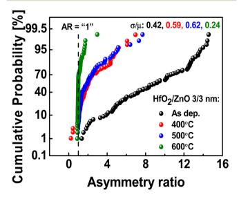
Fig. 9 Cumulative probability of the asymmetry ratio for LTP and LTD behavior in bilayer HfO $_2$ /ZnO synaptic devices without and with thermal annealing from 400 °C to 600 °C for 1 h in an N $_2$  ambient, where the ratio "1" is the ideal state.
