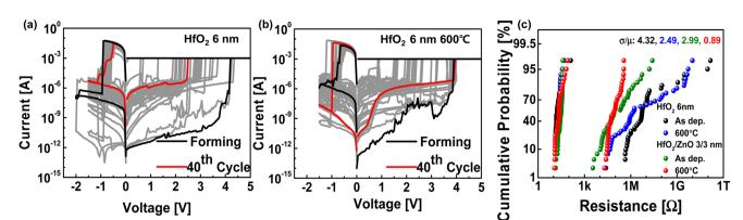
Fig. 7 Typical I-V switching behavior of 6 nm  $HfO_2$  (a) without and with thermal annealing (b) at 600 °C for 1 h in an  $N_2$  ambient compared with that of bilayer  $HfO_2/ZnO$  synaptic devices under the same thermal annealing conditions. (c) Distribution and cumulative probability of the HRS and LRS of  $HfO_2$  (6 nm) and bilayer 3 nm  $HfO_2/3$  nm ZnO synaptic devices without and with thermal annealing.
