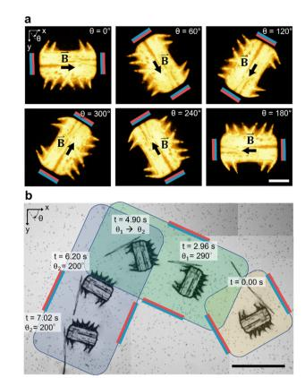
Fig. 4 Magnetic manipulation of a soft polymeric microrobot. (a) Controlled rotational motion of a fluorescent microrobot in a glycerol/ distilled water mixture (50/50 vol%). Scale bar, 100 µm. In the stitched image sequence (b), the navigation of a microrobot along a 90-degree curved pathway using external magnetic field guidance and acoustic propulsion (f = 23.3 kHz,  $V_{PP} = 22.5 \text{ V}$ ) is shown. Scale bar, 500  $\mu\text{m}$ .
