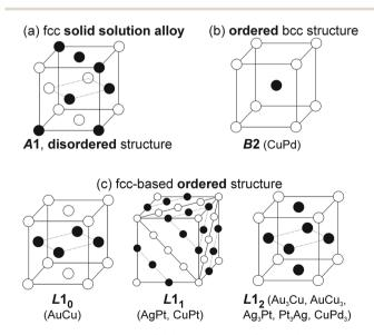
Fig. 5 Crystal structures of (a) SSAs and some (b and c) intermetallics of B2, L1<sub>0</sub>, L1<sub>1</sub>, and L1<sub>2</sub>-typed ordered structures.
