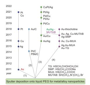
Fig. 3 A decade of development of sputter deposition onto liquid PEG to synthesize metal and alloy NPs and nanoclusters.
