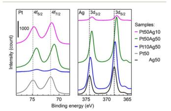
Fig. 10 XPS spectra of Ag/Pt NPs sputtered on Si wafer for 10 s. Dashed lines refer to the reference peak position. Reproduced with permission of ref. 61. Copyright 2021, the American Chemical Society.
