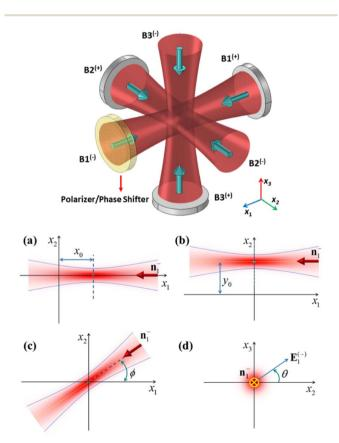
Fig. 1 Schematic diagram of the proposed setup (top diagram) as well as defining the parameters of beam  $\mathbf{1}^{(-)}$  used in the simulations. (a) Axial offset  $(x_0)$ , (b) lateral offset  $(y_0)$ , (c) propagation direction of beam  $1^{(-)}$  with respect to the  $x_1$  axis  $(\phi)$ , and (d) polarization direction of beam  $1^{(-)}$  from the  $x_2$  axis  $(\theta)$ .
