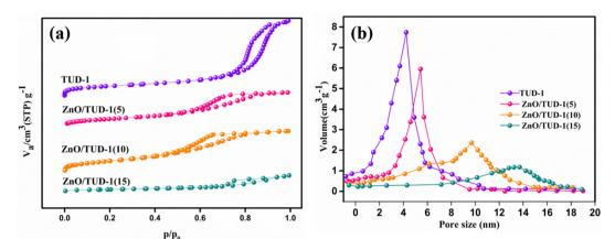
Fig. 7 (a) N<sub>2</sub> adsorption-desorption isotherms and (b) pore size distribution curves of the prepared ZnO/TUD-1(x) nanocomposites.
