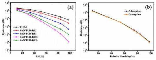
(a) Resistance vs. RH curves for the as-synthesized ZnO/TUD-1(x) nanocomposites and (b) hysteresis curve for ZnO/TUD-1(10)
