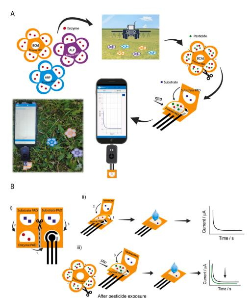
Fig. 7 Schematic representation of (A) flower-like origami paper-based electrochemical biosensor for detecting pesticides using smartphone-assisted potentiostat and (B) device composed of office paper-based screen-printed electrode and three filter pads (i), evaluation procedure of initial enzymatic activity in the absence of pesticide (ii), and residual enzymatic activity after exposure to pesticide solution (iii). Reproduced with permission from ref. 162 Copyright 2022, Elsevier.
