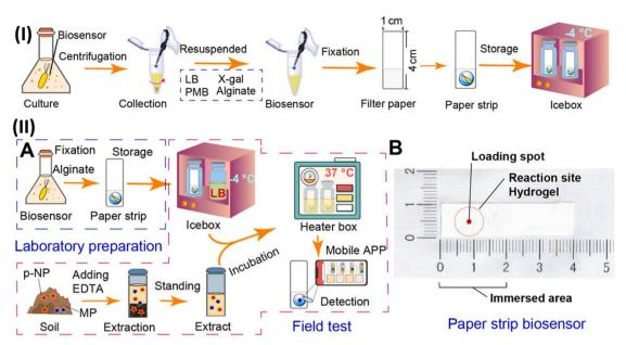
Fig. 8 (I) Schematic illustration of manufacturing of paper-strip biosensor. (II) Diagram of whole-cell biosensor device for detecting MP and pnitrophenol (p-NP): flow-diagram of the fabrication and utilization (A) and objective drawing (B) of whole-cell paper-strip biosensor. Reproduced with permission from ref. 172 Copyright 2023, Elsevier.
