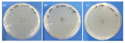
Fig. 11 Reusability: photographs showing the inhibition zone of the reused meltblown fabric coated with MMO-Ag after (a) heating in an oven at 85 °C, (b) exposure to sunlight and (c) UV illumination.
