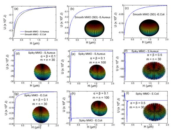
Fig. 8 DLVO interaction energy between MMO and bacteria (*S. aureus* and *E. coli*) using (a) DA approximation and (b)–(i) SEI technique. (a)–(c) are for smooth spheres and (d)–(i) are obtained for spiky MMO with different densities of spikes (m, n) and spike aspect ratios ( $\alpha$ ,  $\beta$ ).
