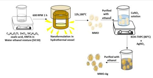
Fig. 1 Schematic diagram of the synthesis procedure for spiky MMO-Ag nanoformulations
