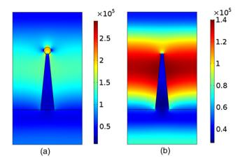
Fig. 13 Simulation results for the magnitude of electric field distribution around a single spike (a) with an Ag nanoparticle and (b) without any Ag
