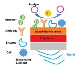
Fig. 1 Components and mechanism of a biosensor.
