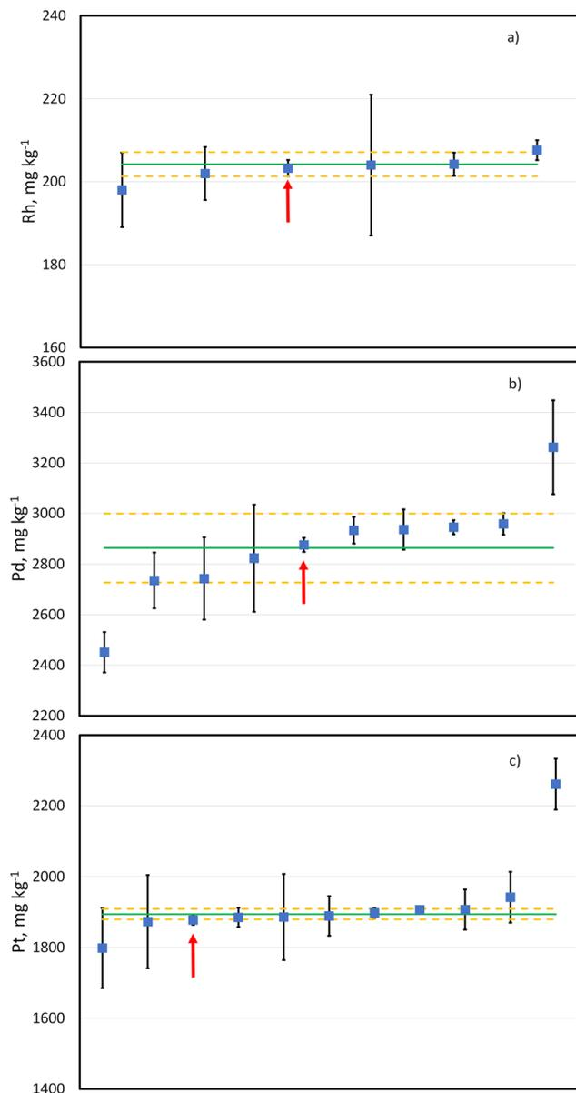
Fig. 5 Mass fractions ( $\text{mg kg}^{-1}$ ) of Rh (a), Pd (b) and Pt (c) in automotive catalyst sample LGC3101. Results submitted for international interlaboratory comparison study CCQM K160 (Platinum Group Elements in Automotive Catalyst). Values obtained in the current study are marked with an arrow. Error bars correspond to combined expanded uncertainties ( $k = 2$ ). Solid line shows the provisional consensus values while dash lines indicate their expanded uncertainties ( $k = 2$ ).
