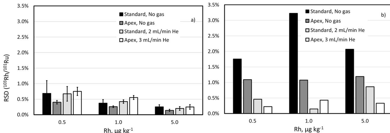
Fig. 3 Precision of ratio  $^{103}\text{Rh}/^{101}\text{Ru}$  for a standard sample introduction system and a desolvating nebuliser (Apex Q) with and without He in the CRC. (a) Internal precision, or RSD of 10 consecutive replicates at 30 s each; (b) external precision, or RSD of 3 measurements of the same sample about 1 h apart (each measurement consisting of 10 consecutive replicates at 30 s each). Ruthenium is added as an IS so that  $^{103}\text{Rh}/^{101}\text{Ru}$  is close to 1 : 1.
