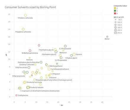
Fig. 6 An example plot of  $\delta_P$  vs.  $\delta_H$  sized by boiling point for consumer solvents (white spirit omitted, as no one single  $\delta_H$  or  $\delta_P$  value).
