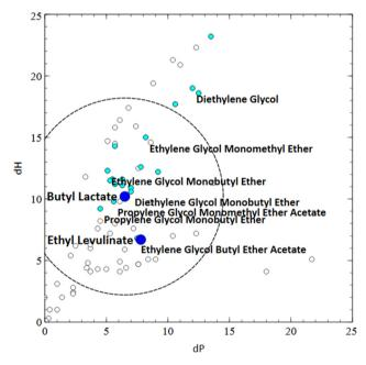
Fig. 10 Butyl lactate (4, dark blue circle) and ethyl levulinate (5) in 2D Hansen space ( $\delta_H$  vs.  $\delta_P$ ) in comparison to glycol ether solvents (light blue circles) and the wider group of paint solvents (unfilled circles). The large dotted circle shows a radius of 8, typical of the  $\theta$ -solvent radius of a polymer.
