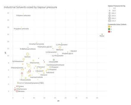
**Fig. 5** An example plot of  $\delta_P$  vs.  $\delta_H$  sized by vapour pressure for industrial solvents.
