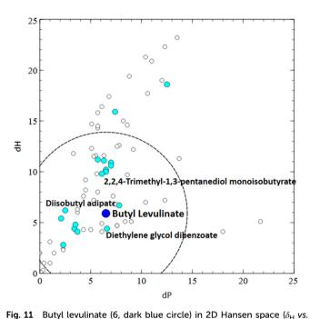
$\delta_{\rm P}$ ) in comparison to coalescent solvents (light blue circles) and the wider group of paint solvents (unfilled circles). The large dotted circle shows a radius of 8, typical of the  $\theta$ -solvent radius of a polymer.
