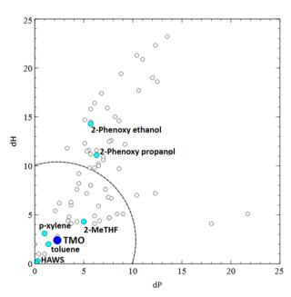
Fig. 9 TMO (3, dark blue circle) in 2D Hansen space  $(\delta_{\rm H} \ vs. \ \delta_{\rm P})$  in comparison to aromatic solvents (light blue circles) and the wider group of paint solvents (unfilled circles). The large dotted circle shows a radius of 8, typical of the  $\theta$ -solvent radius of a polymer. (HAWS = High aromatic white spirit).
