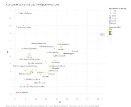
Fig. 4 An example plot of  $\delta_P$  vs.  $\delta_H$  sized by vapour pressure for consumer solvents (white spirit omitted, as no one single  $\delta_H$  or  $\delta_P$  value).
