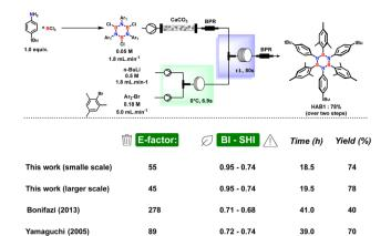
**Fig. 6** Comparison of *E*-factor, benign–safety/hazard index, reaction time and yields for this work in flow and other procedures in batch conditions.
