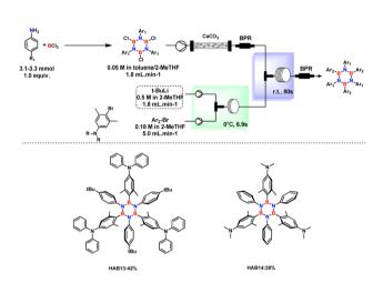
Fig. 5 Synthesis of aminated HABs under continuous flow conditions. Reaction conditions: Ar–Br (0.18 M in 2-MeTHF) t-BuLi (0.5 M in pentane/2-MeTHF), and TCB solution (0.05 M in toluene/heptane/2-MeTHF) produced from aniline derivatives (1.0 equiv.); BCl $_3$  (1.2 equiv.) were introduced to the flow system fabricated by PEEK Tee (ID: 0.5 mm) and PTFE tube ( $\emptyset$ i.d.: 1 mm) using a high-pressure syringe pump.
