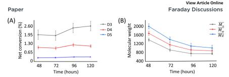
Fig. 5 Plots of (A) net conversion of the cyclic oligomers against time and (B) the molecular weight of the linear polymer. Net conversion = conversion from enzyme-catalysed reaction minus conversion from negative control reaction.
