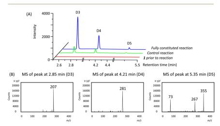
**Fig. 4** Gas chromatograms (A) and mass spectra (B) of the reaction mixtures for substrate **1**. The fragmentation patterns of D3, D4 and D5 are consistent with the electron ionisation fragmentation patterns observed for authentic standards.
