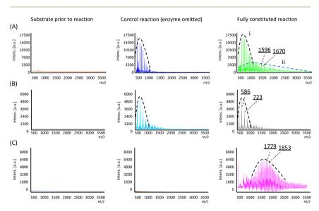
Fig. 3 MALDI mass spectra of the products of the polymerisation reactions for substrate 1 (A), 2 (B), 3 (C) with population distributions indicated. Illustrative m/z values are also shown, the difference of which corresponds to a Si(Me)<sub>2</sub>O or SiMePhO repeating unit.
