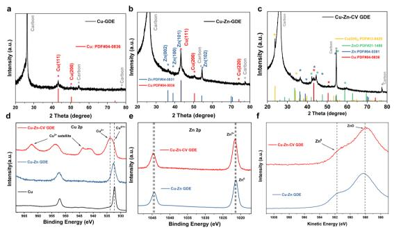
Fig. 3 XRD patterns of (a) Cu-GDE, (b) Cu-Zn-GDE and (c) Cu-Zn-CV-GDE catalysts. (d) Cu 2p XPS spectra of Cu-GDE, Cu-Zn-GDE and Cu-Zn-CV-GDE catalysts. GDE catalysts. (e) Corresponding Zn 2p XPS spectra of Cu-Zn-GDE and Cu-Zn-CV-GDE catalysts. (f) Zn LMM spectra of Cu-Zn-GDE and Cu-Zn-CV-GDE catalysts
