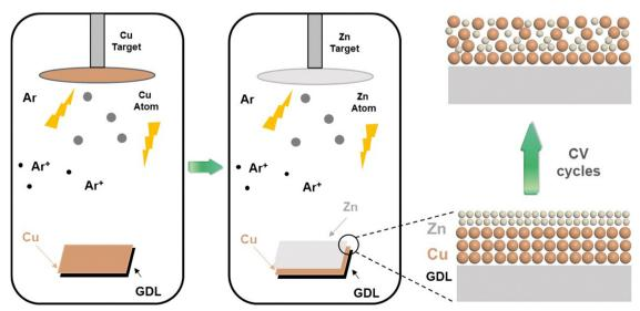
Fig. 1 Schematic diagram of the preparation process of the bimetallic catalysts on the GDL.
