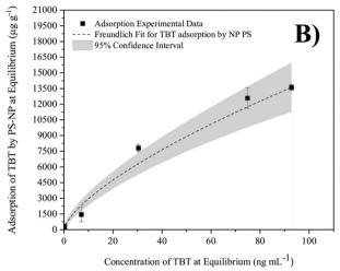
Fig. 2 Adsorption of TBT by large PS-NP in pH 8 Milli-Q water, showing Freundlich fitting for TBT adsorption in phosphate pH 8 Milli-Q buffer across A) an extended concentration range and B) a concentration range limited by the TBT solubility limit.
