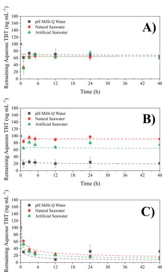
Fig. 1 Kinetics of TBT adsorption by PS-NP, showing the relationship between aqueous TBT concentration (ng  $\mbox{mL}^{-1}$  TBT) and time (h) during kinetics experiments. A) Large PS-NP, B) medium PS-NP and C) small PS-NP. Experimental replicates are represented with error bars (SD, n = 3).
