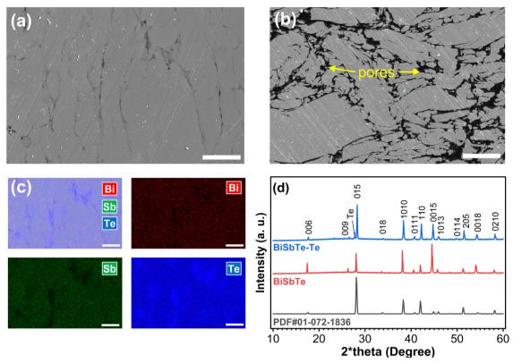
Fig. 2 Scanning electron microscopy (SEM) images of the cross-section of (a) BiSbTe-Te (scale bar: 5 μm). (b) BiSbTe (scale bar: 5 μm) and (c) EDS elemental mapping of BiSbTe-Te (scale bar: 5 μm). (d) X-ray diffraction results of BiSbTe and BiSbTe-Te. The reference XRD curve at the bottom is for Bi<sub>0.4</sub>Sb<sub>1.6</sub>Te<sub>3</sub> obtained from the ICSD (inorganic crystal structure database).
