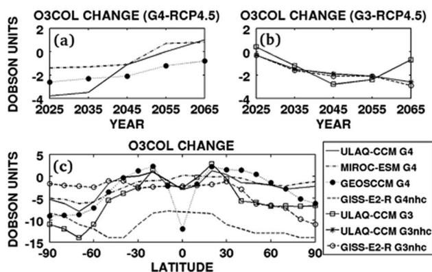
Fig. 8 Modeling simulations of global O<sub>3</sub> column changes in (a) G4 and (b) G3 with respect to the base case RCP4.5 over time. (c) Zonally and time-averaged column ozone changes (2040–2049). Reprinted with permission of the publisher from Pitari *et al.*, *J. Geophys. Res.*, 2014, 119, 2629–2653.
