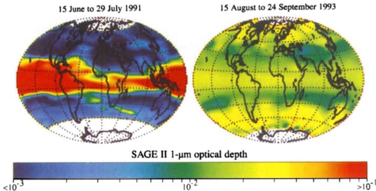
Fig. 3 Stratospheric aerosol optical depth, measured by the stratospheric aerosol and gas experiments-II (SAGE II), was observed to confine in the tropics immediately after Mt. Pinatubo's eruption in June 1991 (left), before the aerosols were dispersed two years later (right). Reprinted with permission of the publisher from McCormick *et al.*, *Nature*, 1995, 373, 399–404.
