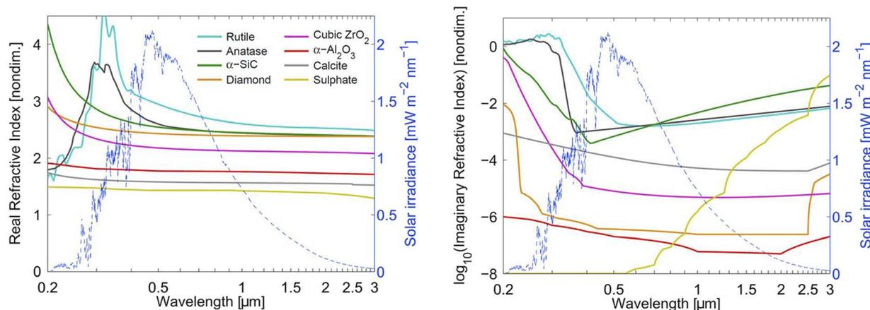
Fig. 4 Shortwave real (left) and imaginary (right) refractive index of different aerosol types based on both available experimental data and estimates from model dielectric functions. Reprinted with permission of the publisher from Dykema *et al.*, *Geophys. Res. Lett.*, 2016, **43**, 7758–7766.
