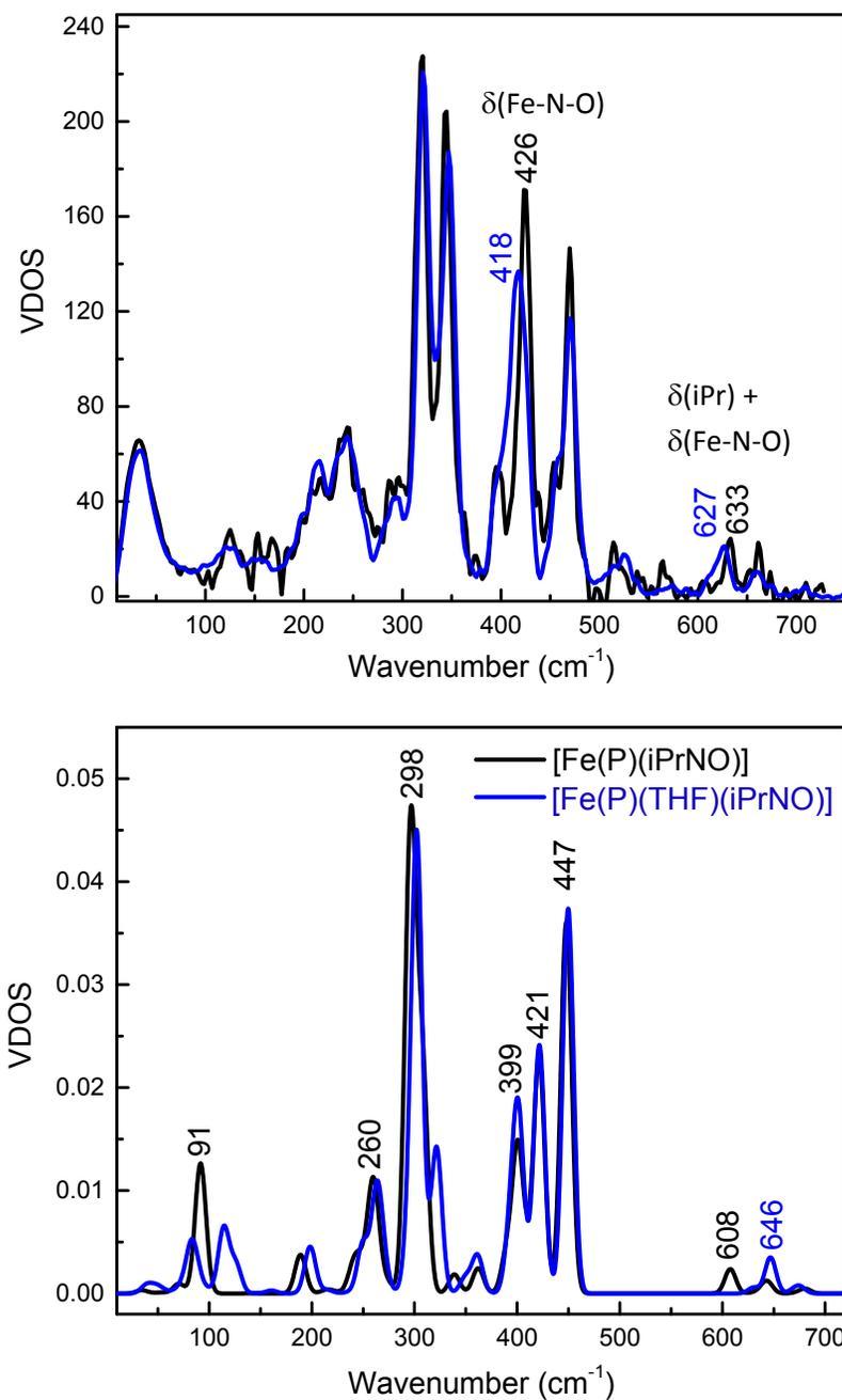
**Figure 7.** Top: NRVS-derived vibrational density of states (VDOS) for [<sup>57</sup>Fe(TPP)(THF)(iPrNO)] (black) and the <sup>15</sup>N-labeled iPrNO complex (blue). Bottom: BP86/TZVP calculated NRVS VDOS for [Fe(P)(iPrNO)] (black; P<sup>2-</sup> = porphine dianion) and [Fe(P)(THF)(iPrNO)] (blue).
