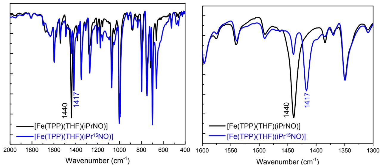
**Figure 3.** Left: Overlay of the IR spectra of [Fe(TPP)(THF)(iPrNO)] (black) and of the <sup>15</sup>N-labeled complex, [Fe(TPP)(THF)(iPr<sup>15</sup>N)] (blue). The data were obtained in KBr pellets. Right: Expanded region of the N-O stretching frequency. The natural abundance isotopes (n.a.i.) complex [Fe(TPP)(THF)(iPrNO)] has one isotope sensitive feature at 1440 cm<sup>-1</sup> that shifts to 1417 cm<sup>-1</sup> upon <sup>15</sup>N-labeling.
