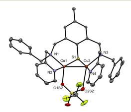
Fig. 3 ORTEP diagram (30% probability) for the dicationic unit of 6. H-atoms are omitted for clarity. Selected bond distances (Å): Cu1-Cu2 2.5475(5), Cu1-S1 2.1798(8), Cu2-S1 2.1661(8), Cu1-N1 2.043(2), Cu1-N2 1.959(3), Cu1-O1S2 2.176(2), Cu2-N3 2.114(3), Cu2-N4 1.945(3), Cu2-O2S2 2.674(9); see Tables S1-S3, ESI.†
