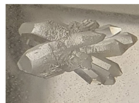
Fig. 1 Single N 2 O 5 crystal cluster from the current work. This cluster was 1.2 cm across at its longest point.
