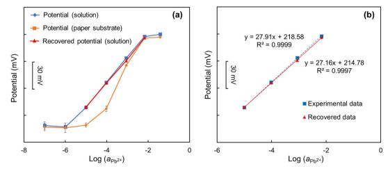
Fig. 6 Corrective protocol to predict interference free sensor response from the paper-based potential in case 2: (a) calibration curves of the fabricated Pb<sup>2+</sup> ISEs on paper substrate, on standard mixed solution and recovered solution-based calibration curve from paper-based calibration curve; (b) slopes and linearities of the experimental solution-based calibration curve and the recovered solution-based calibration curve.
