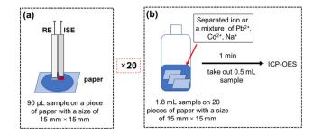
Fig. 1 (a) Conventional paper-based microfluidic solution sampling coupled with potentiometric cell; (b) protocol for determining the adsorption of heavy metal ions onto the paper substrates.
