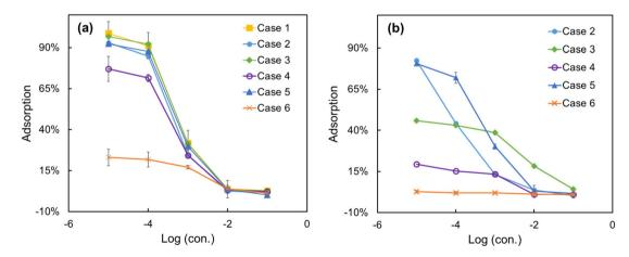
Fig. 5 Adsorption of (a) the primary ions and (b) the interfering ions on paper substrate during the potentiometric measurement with ISEs. The primary ion in cases 1–6 is Pb<sup>2+</sup>; the interfering ions are Cd<sup>2+</sup> or Na<sup>+</sup> with various concentrations (Table S1†).
