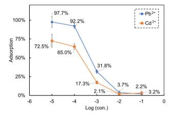
Fig. 2 Adsorption of Pb<sup>2+</sup> and Cd<sup>2+</sup> onto the paper substrates during paper-based potentiometric measurements in pure samples containing a single ion concentration.
