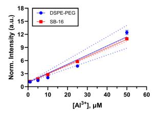
Fig. 2 Response of the Al<sup>3+</sup> sensors made with DSPE-PEG and SB-16 to analyte ranging from 1  $\mu M$  to 50  $\mu M$ . While there is a small variation, both responses show a similar trend (two-tailed t-test, 95% C.I, p = 0.1134 > 0.05). Note, the data was normalized to the response at 1  $\mu$ M, also where not visible the errors bars are smaller than the data points (n = 3).
