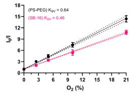
Fig. 4 Stern–Volmer response from the  $O_2$  sensors fabricated using FNP at varying  $O_2$  concentrations. The sensors made with PS-PEG show a more sensitive response to changes in oxygen than its SB-16 counterpart (statistical difference verified *via* two-tailed *t*-test, 95% C.I., p = 0.0037 < 0.05). Both sensors were excited at 405 nm and the emissions observed 650 nm. Where not visible the error bars are smaller than those of the data points (n = 3).
