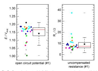
Fig. 3 Open circuit potentials (left) and uncompensated resistance (right) of the activated standard electrodes (100  $\mu g$  cm $^{-2}$  nickel–cobalt–oxide nanopowder). Measurements were performed by 11 different laboratories/experimenters, indicated by different colors. The box plot representation is explained in the text.
