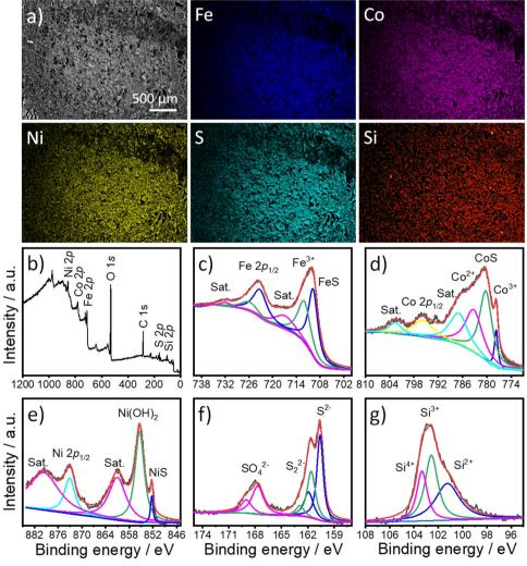
Fig. 3 (a) Top-view SEM and the corresponding atoms (Fe, Co, Ni, S, and Si) mapping images of FCNSSi on carbon paper electrode. (b) Wide scan XPS survey of FCNSSi powder and high-resolution XPS spectra of (c) Fe 2p, (d) Co 2p, (e) Ni 2p, (f) S 2p, and (g) Si 2p orbitals.
