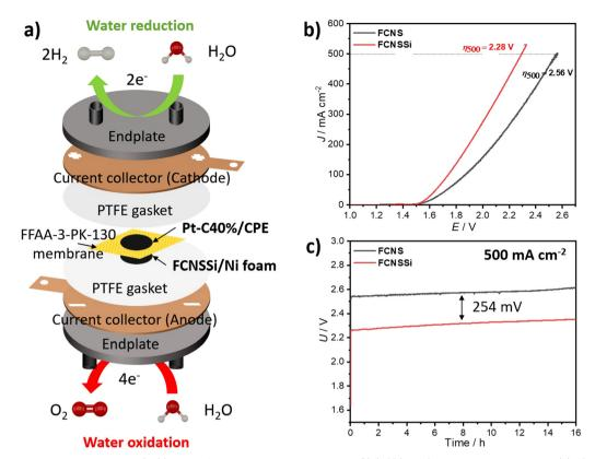
Fig. 9 (a) Zero-gap cell assembly using FCNSSi on Ni foam at anodic side against Pt/C (40%) on CPE at cathodic side, and (b) LSV measurements, and (c) chronopotentiometry test at 500 mA cm<sup>-2</sup> for 16 h of both pristine FCNS and FCNSSi on Ni foam electrodes.
