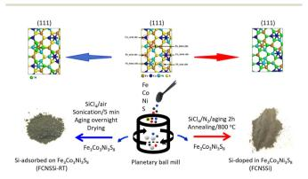
Fig. 1 Schematic illustration of the synthetic pathway of Si-doped in trimetallic pentlandite (FCNSSi) and Si-adsorbed at trimetallic pentlandite (FCNSSi-RT) surface.
