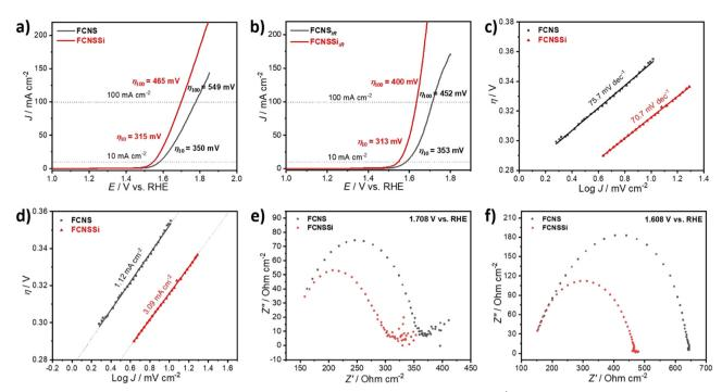
Fig. 4 LSV curves (a) before and (b) after iR compensation in 1.0 M KOH solution at scan rate of 10 mV s<sup>-1</sup>, (c) derived Tafel plots from LSV curves, (d) the estimated exchange current density  $(J_0)$ , and EIS at (e) 1.708 V vs. RHE and (f) 1.608 V vs. RHE of our materials on glassy carbon electrode
