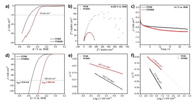
Fig. 7 (a) LSV curves of the as-prepared FCNS and FCNSSi in 0.5 M  $H_2SO_4$  solution at scan rate of 50 mV  $s^{-1}$ , (b) EIS at -0.255 vs. RHE, (c) chronoamperometry test at -0.1 vs. RHE, (d) LSV curves after HER performance for 24 h, (e and f) the derived Tafel plots and the estimated exchange current density ( $J_0$ ), respectively, of FCNS and FCNSSi samples on glassy carbon electrode.
