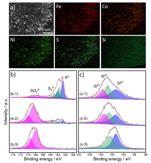
Fig. 5 (a) Top-view SEM and the corresponding atoms mapping (Fe, Co, Ni, S, and Si) images of FCNSSi on carbon paper electrode after chronopotentiometry test at 100 mA cm<sup>-2</sup> for 24 h. High resolution XPS spectra of (b) S 2p and (c) Si 2p orbitals of (b-1 and c-1) the prepared electrode, and after (b-2 and c-2) 1 h and (b-3 and c-3) 24 h OER.
