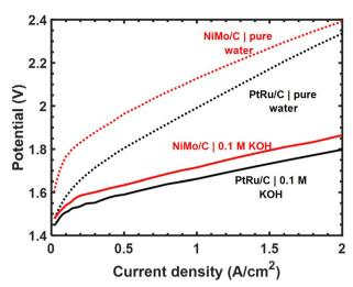
Fig. 4 Polarization data for full HEM electrolysis using 25 wt% Ni-Mo/o-C and Pt-Ru/C (50 wt% Pt, 25 wt% Ru) cathodes using aryl-ammonium based membrane/binder polymers and IrOx anode catalysts. The total catalyst loading of Ni-Mo/oC was 1 mg<sub>cat</sub> cm<sup>-2</sup> and for Pt-Ru/C it was 0.15 mg<sub>cat</sub> cm<sup>-2</sup>. Unsupported IrO<sub>x</sub> nanoparticle anodes were loaded at  $3 \text{ mg}_{\text{cat}} \text{ cm}^{-2}$ .
