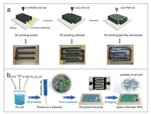
Fig. 8 3D printing technology for the fabrication of PMSCs. (a) G-VNQDs/GO anode,  $V_2O_5/GO$  cathode and LiCl-PVA gel-like electrolyte constructed with the 3D printing method. Reproduced with permission.<sup>97</sup> Copyright 2018, Wiley-VCH. (b) Schematic illustration of the ionogel-based quasi-solidstate MSC. Reproduced with permission. 98 Copyright 2020, Wiley-VCH.
