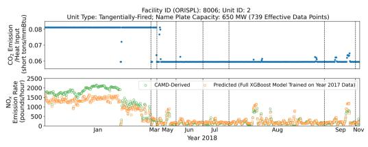
Fig. 7 The ratios between  $CO_2$  emissions and heat input (upper), and CAMD-derived *versus* predicted  $NO_x$  emission rates (bottom,  $R^2 = 0.86$ ) from Unit 2 of the Roseton Generating LLC facility in Newburgh, NY (Facility ID: 8006) in 2018, with abnormal high  $NO_x$  emission rates in January corresponded with the under-prediction zone shown in the left scatter plot in Fig. 5a.
