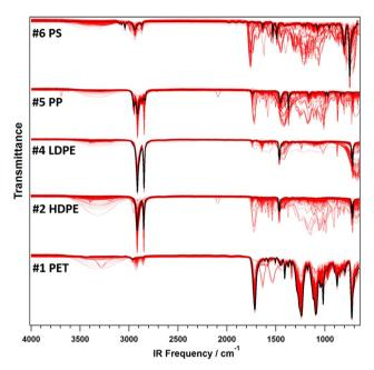
Fig. 2 Mid-infrared (4000–650 cm<sup>-1</sup>) spectra of 835 postconsumer plastics that were evaluated in this study (red). Virgin polymer (black). Spectra are shown in percent transmittance (y-axis minimum is 30% per RIC).
