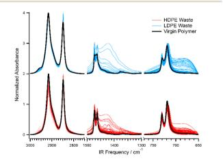
**Fig. 4** Semicrystalline regions of HDPE (red) and LDPE (blue) waste plastics. Reference HDPE and LDPE spectrum (black).
