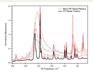
Fig. 5 Polypropylene waste plastic with zero carbon black content (black). Black-colored polypropylene waste plastics (red). Spectra were normalized to the 2916 cm<sup>-1</sup> asymmetric methylene stretch.
