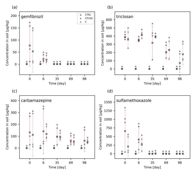
Fig. 2 Concentration of (a) gemfibrozil, (b) triclosan, (c) carbamazepine, and (d) sulfamethoxazole in control (CTRL), chemical contaminants + 100 mg HDPE microplastic  $kg^{-1}$  soil (CP100), and chemical contaminants (C) treated soils. For each time point, treatments with the same letter have no significant difference between them. Markers represent individual samples. Grey squares represent the means. Error bars show  $2 \times$  the standard error of the mean.
